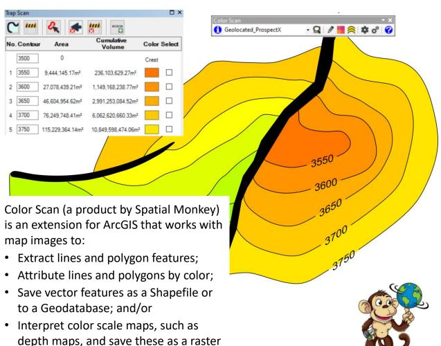
Color Scan also features Trap Scan, which extracts depth/area pairs from prospect and leads maps, such that these values can be loaded into QwikEval in Player.
